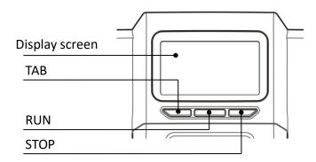
Display screen: Operate by touch screen or mouse which connect with USB
